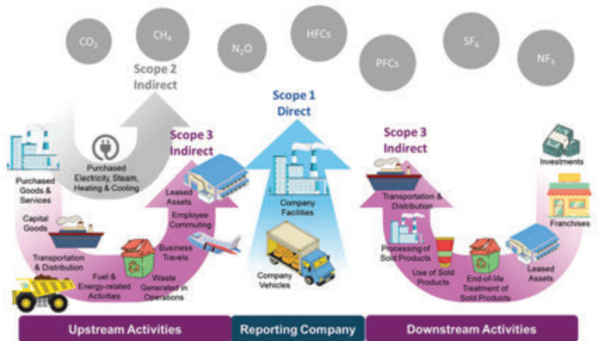
Schematic overview of greenhouse gas (GHG) emissions across Scopes 1, 2, and 3 as defined by the GHG Protocol covered by our Carbon Accounting & Management Platform
