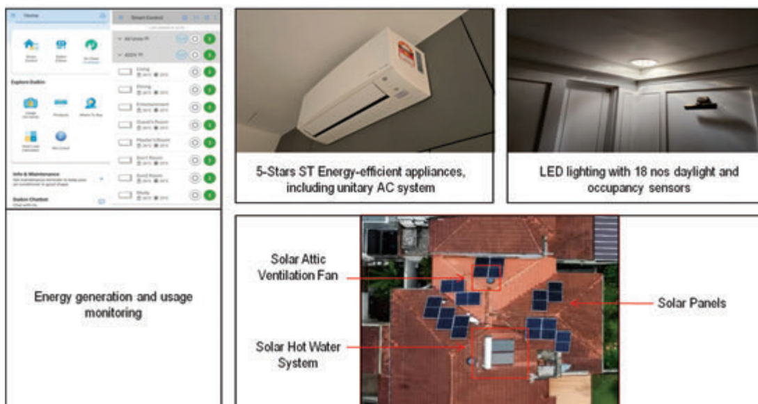
Figure 2: Active designs incorporated into Danau Villa
