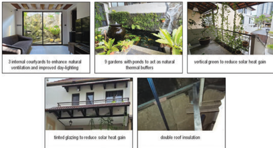
Figure 1: Passive designs incorporated into Danau Villa
