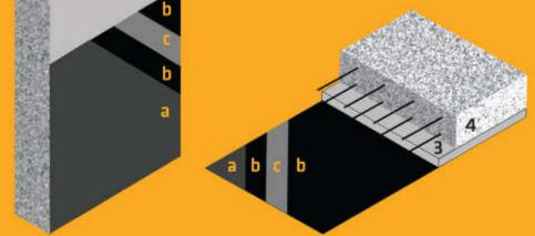
SikaBit® W-15 is a sheet membrane waterproofing system consisting of a cross laminated HDPE carrier film laminated with a modified bitumen based adhesive on both surfaces. Due to the double-sided structure the SikaBit® W-15 system can be installed single or (partially) double layered and does not require any accessories such as tapes and pastes etc.
