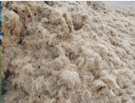
SHORT LOOSE FIBRE AS BOILER FUEL
