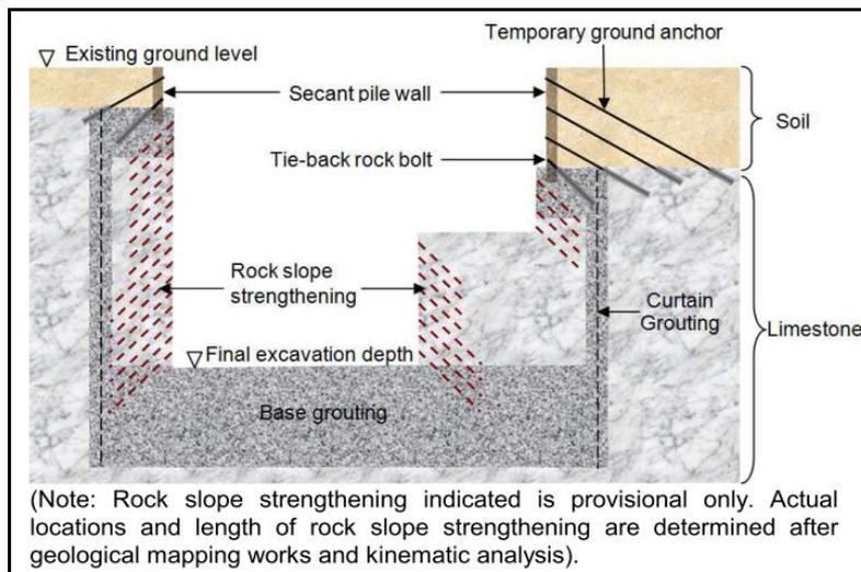
**Figure 2: Schematic of excavation works**
