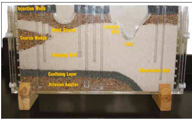
Figure 4: A sand tank model Source: University of Nebraska-Lincoln (2009)
