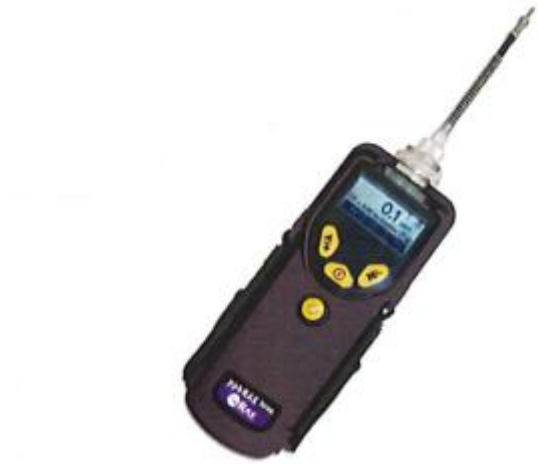
Figure 4: VOC Detector ppbRAE 3000+
