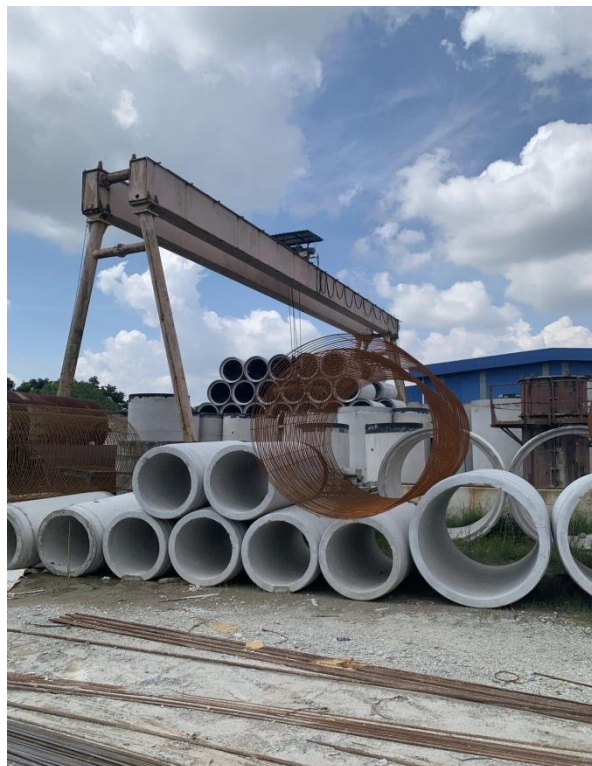
Figure 7: Finished jacking pipes and reinforcement cages at the factory stockyard, served by overhead gantry cranes
