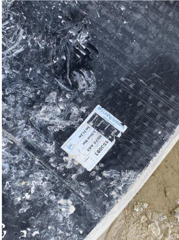
Figure 8: Sample roll of HDPE lining sheet with manufacturer's identification label
