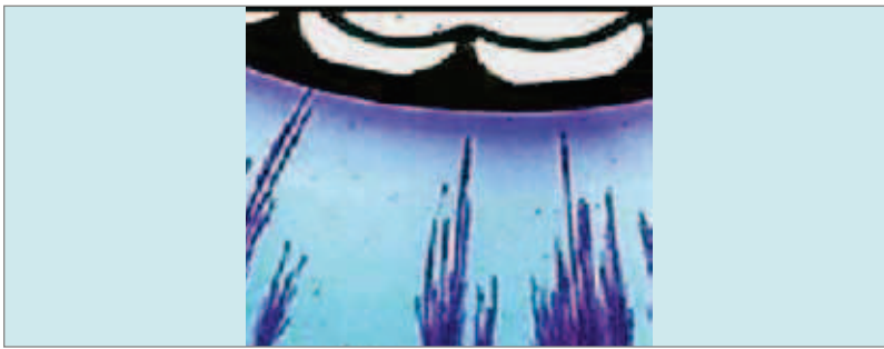
Figure 1: Typical Water Tree in Power Cables
