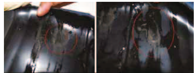
Figure 3: Burn mark at the insulation (Y-phase).
