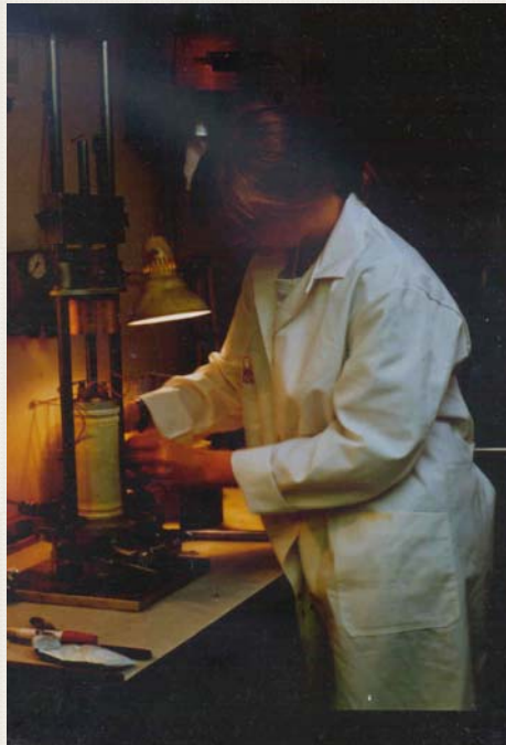
Building in of triaxial sample in NGI's laboratory
