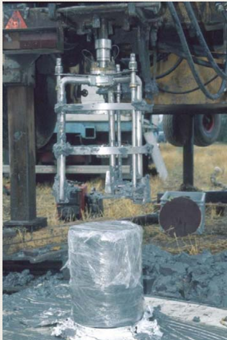
Block sample cleaned and wrapped in plastic cling film
