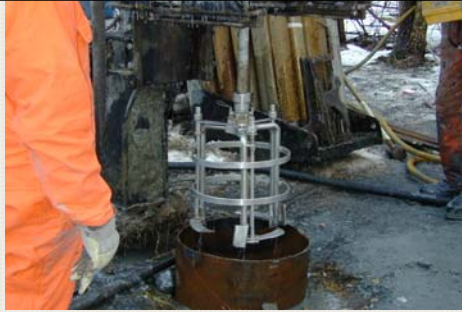
Sampler is lowered into borehole
