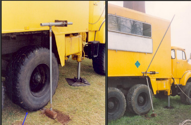
Normal force applied to beam for good contact with ground surface
