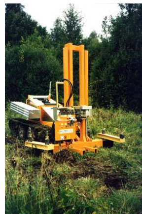
Geotech simple rig
