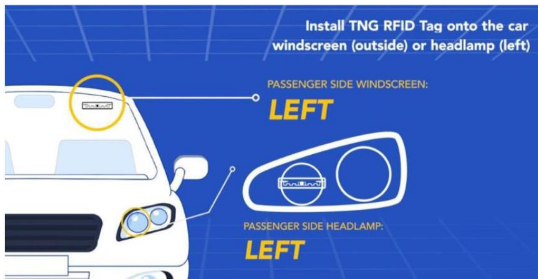
Figure 1: Install TNG RFID Tag onto car's windscreen or headlamp.
