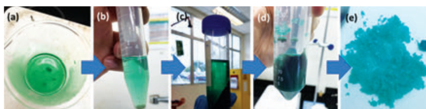
Figure 2: (a) Ni solution recovered from spent catalysts, with the presence of some additional impurities. (b) Separation of solvent and precipitates after centrifugation. (c) Concentrated Ni solution. (d) Post drying and crystallisation. (e) Nickel sulphate crystals.
