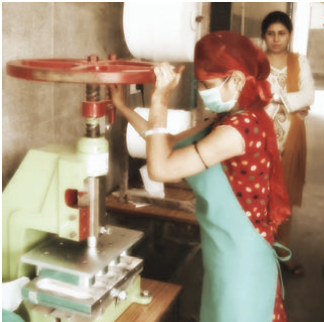
Figure 2: Hand pressing the sanitary pads (Adopted from https://www.aakarinnovations.com/mini-factories )
