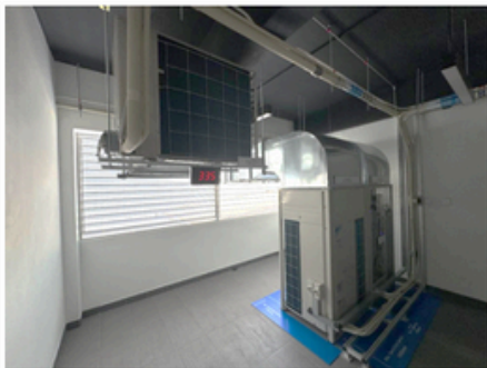
LOUVER DESIGN – TO SIMULATE AC PERFORMANCE vs LOUVER OPENING
