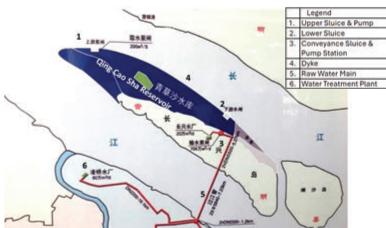
Figure 3: Layout plan of Qing Cao Sha 7,190 Mld Scheme in Shanghai
