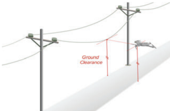
Figure 5: Ground clearance measurement by using UAS
