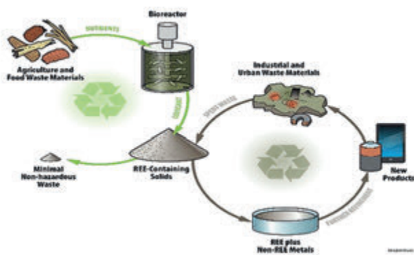
Figure 4: Conceptual scheme of bioleaching in REE (Jin et al. , 2019)
