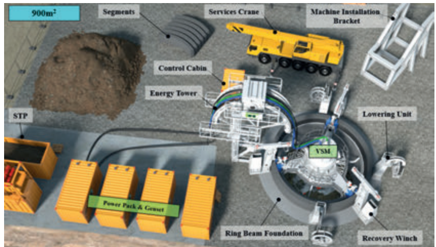
Figure 2: Typical compact site laydown using VSM construction method
