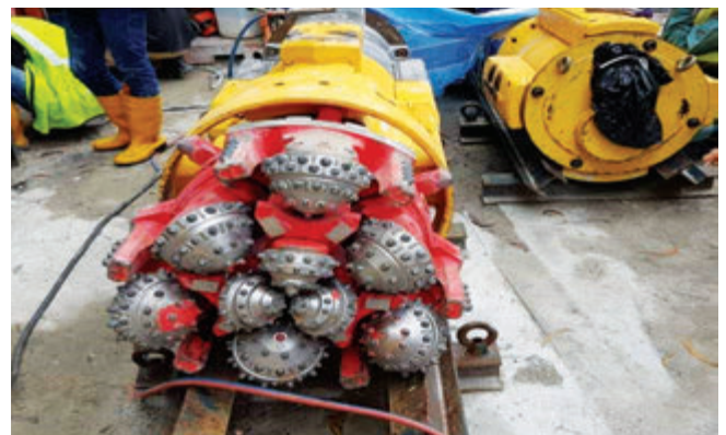
Figure 3.0: Pressurised slurry removal method for curve drive (nominal diameter 250-700mm narrow pipe driving method), ACEMOLE
