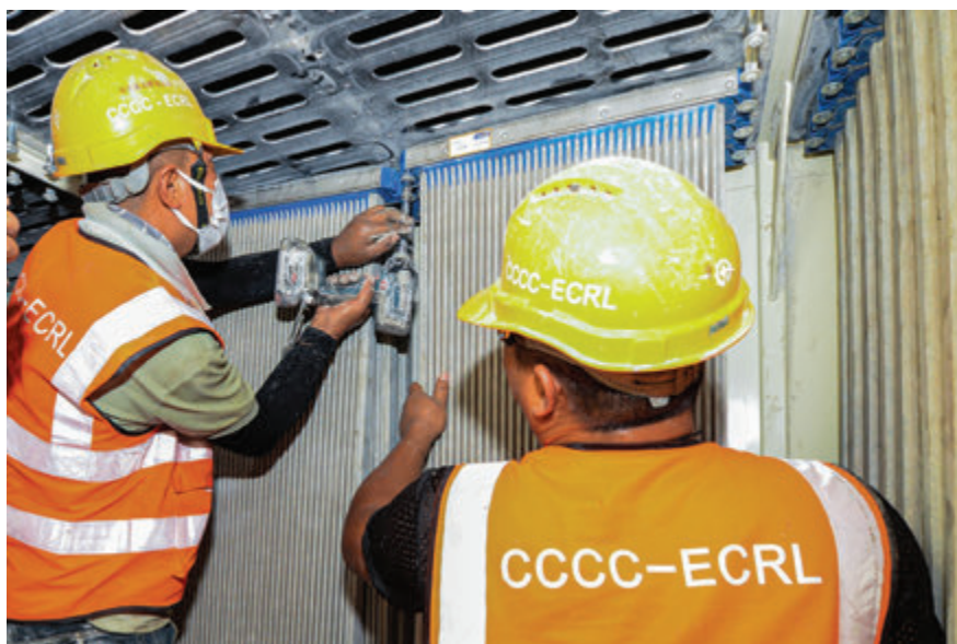
Workers installing dust collector filter elements inside the TBM1
