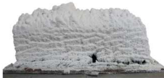
Intumescent coating exposed to a fire – demonstration of thermal increase
