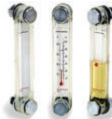
The oil level in the hydraulic tank should also be read frequently to ensure it is correct. If it drops too low due to leakage, the system will not work efficiently. It is estimated that the loss of one drop per second will add up to 1,500 litres of oil lost in a year. The low oil level can cause a vortex in the reservoir. Subsequently, air trapped in the pump inlet will cause dangerous fluctuations and unbalanced pressure on system.
