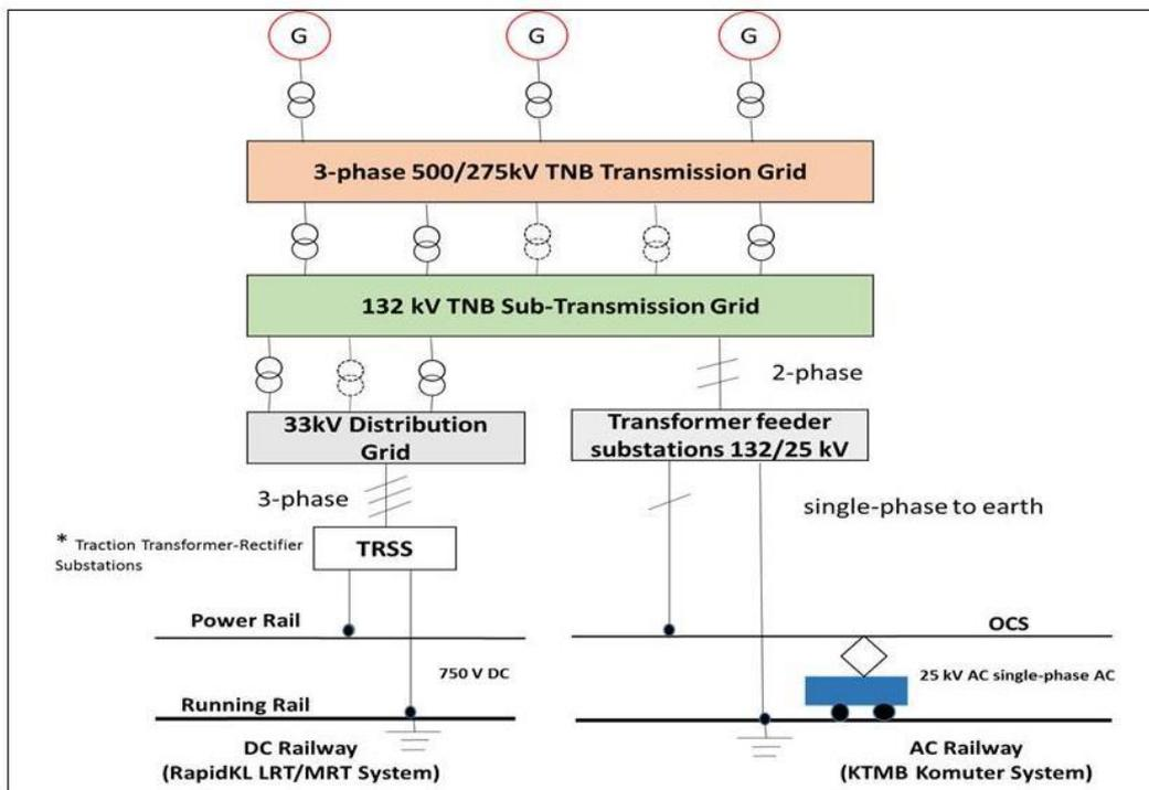
**Figure A2: Structure of Traction Power Supply System for Malaysia’s Electric Railways**
