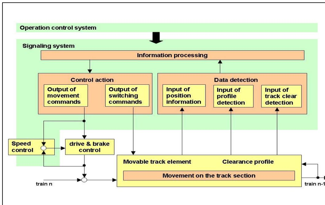
**Figure A3: Processes of Railway Signalling System for Safe Control of Rail Traffic Movements**
