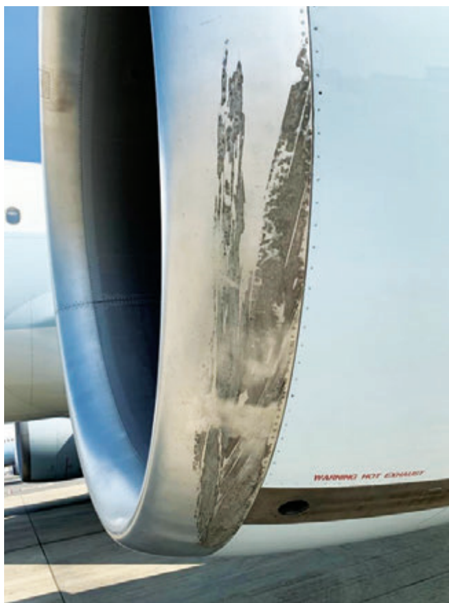
Figure 3: Typical corrosion on the air inlet lip skin
