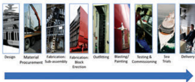
Figure 1: Generic shipbuilding process (Courtesy of OMAHAMS Corp)
