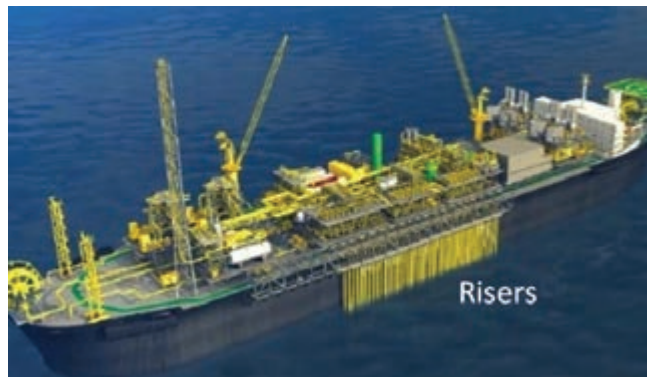
Figure 4: Risers connected to the side of the FPSO in lieu of the turrets [Reference 6]
