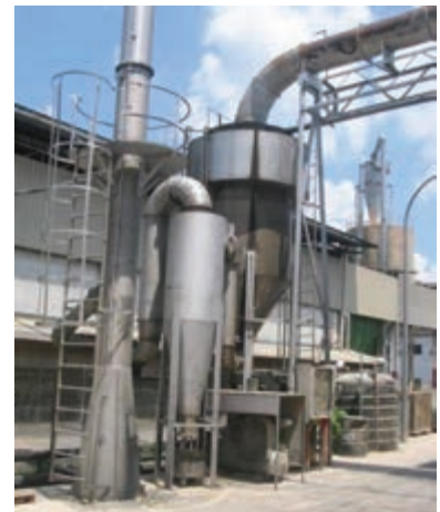
JOINT DISPOSAL OF WASTE WOOD AND WASTEWATER BY INCINERATION AND EVAPORATION
