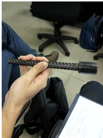
A Moment® JoinTec Coupler Mounted on Threaded Steel Bar
