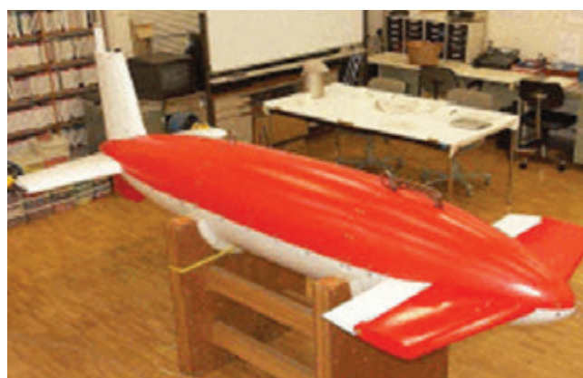
Figure 15: AUV that was used as a towed vehicle [16]
