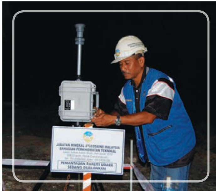
24-hour dust monitoring near residence using High Volume sampler (HVS)
