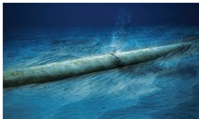
Leak caused by crack in subsea pipeline
