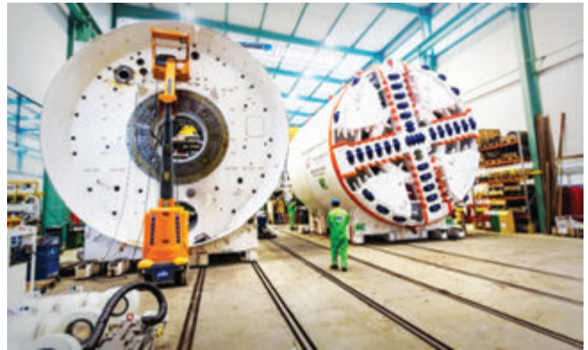
MRT Line 1 Tunnel Boring Machine under construction
