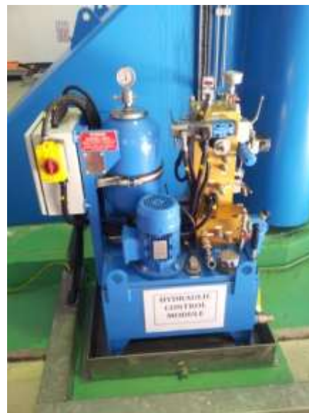
Figure 6: Hydraulic control module
