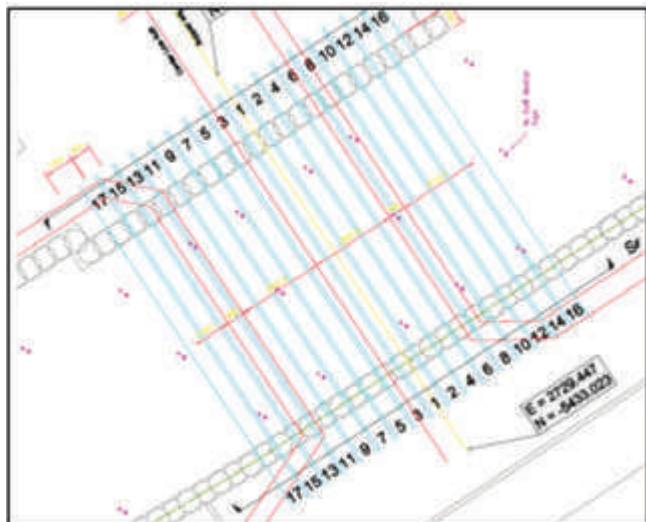
Figure 11: Position of 18 settlement markers along Jalan Cheras
