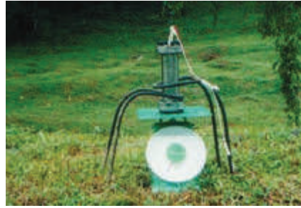
Figure 5.3: Early thrust measurement method.
