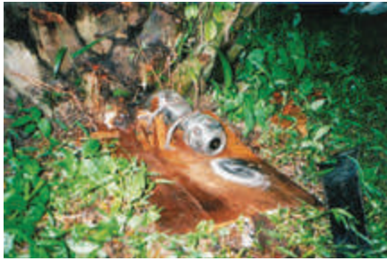
Figure 5.2: Testing the rocket motor shielded by oil palms.
