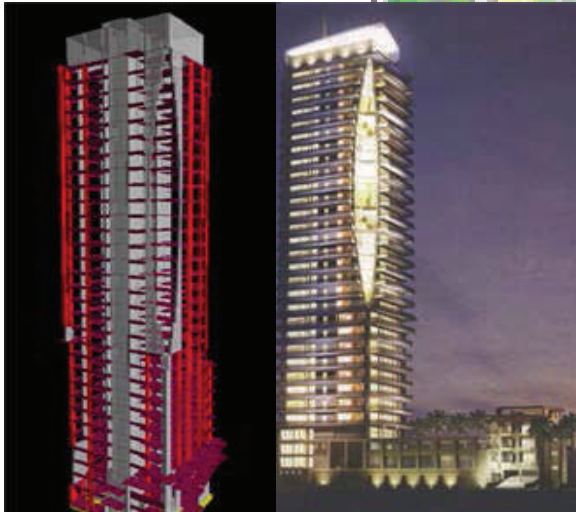
RAM Structural System Building model
