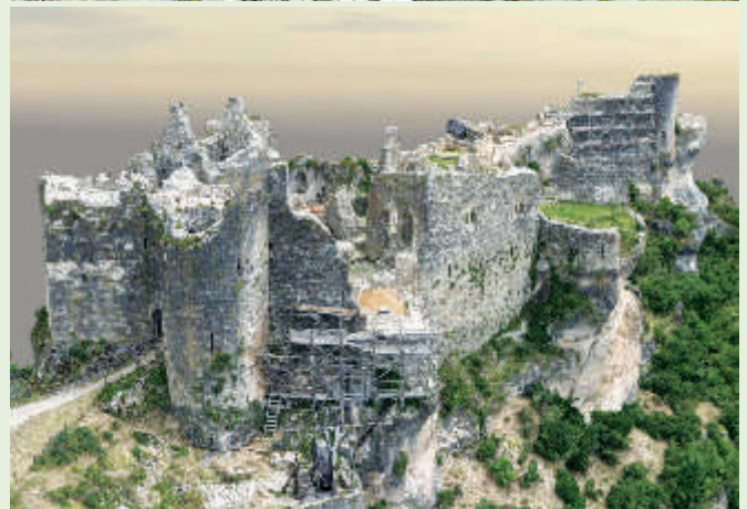
In addition to requiring much less labor and expensive hardware to acquire, the 3D photogrammetric reconstructions are much more visually understandable than point clouds while being light enough to view in a web browser.
