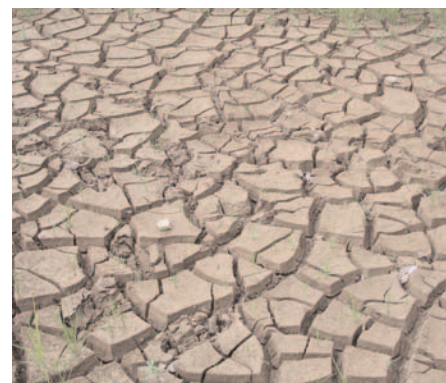
Figure 5 : Typical slime in ex-mining land. Looks solid but is very soft just below the surface.
