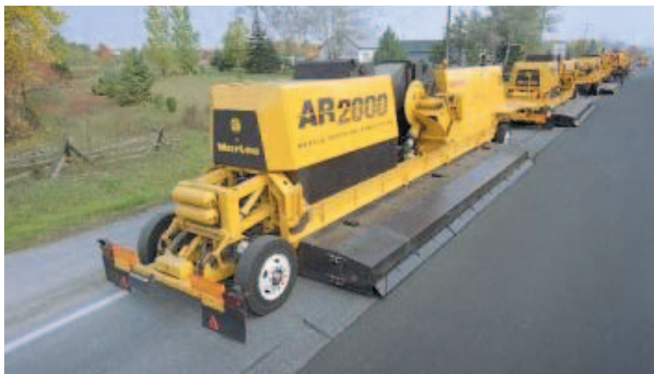
Figure 2: HIPR machine using combination of hot air under forced convection and low level infra-red heating system [2]
