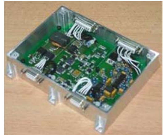
Figure 4: Battery charge regulator
