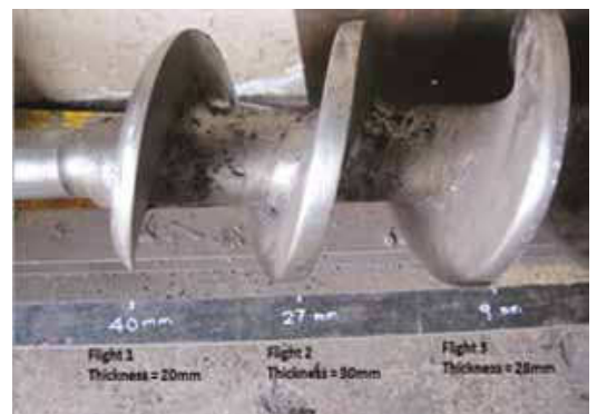
Photo 2: Abrasion wear of P20 screw press
