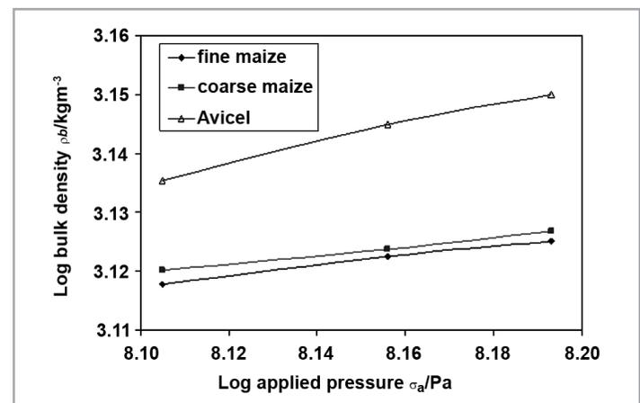
Figure 6: Log bulk density as a function of log applied pressure. The lines are the trend lines
