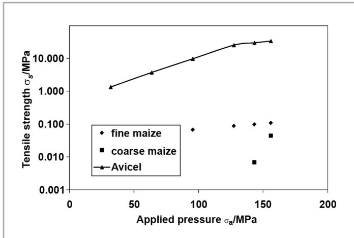
Figure 8: Tensile strength as a function of applied pressure. The line is the trend line
