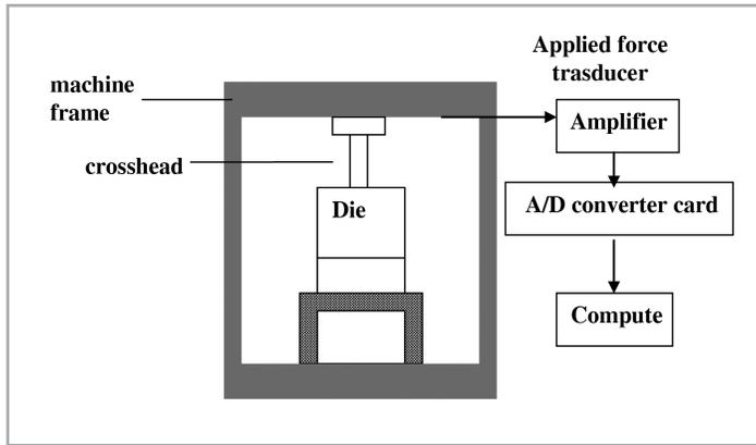
Figure 3: Schematic layout of the uniaxial die compaction system
