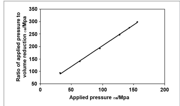
Figure 5: Experimental data fitting into Kawakita and Lüdde (1970/71) equation for fine maize powder at ambient conditions
