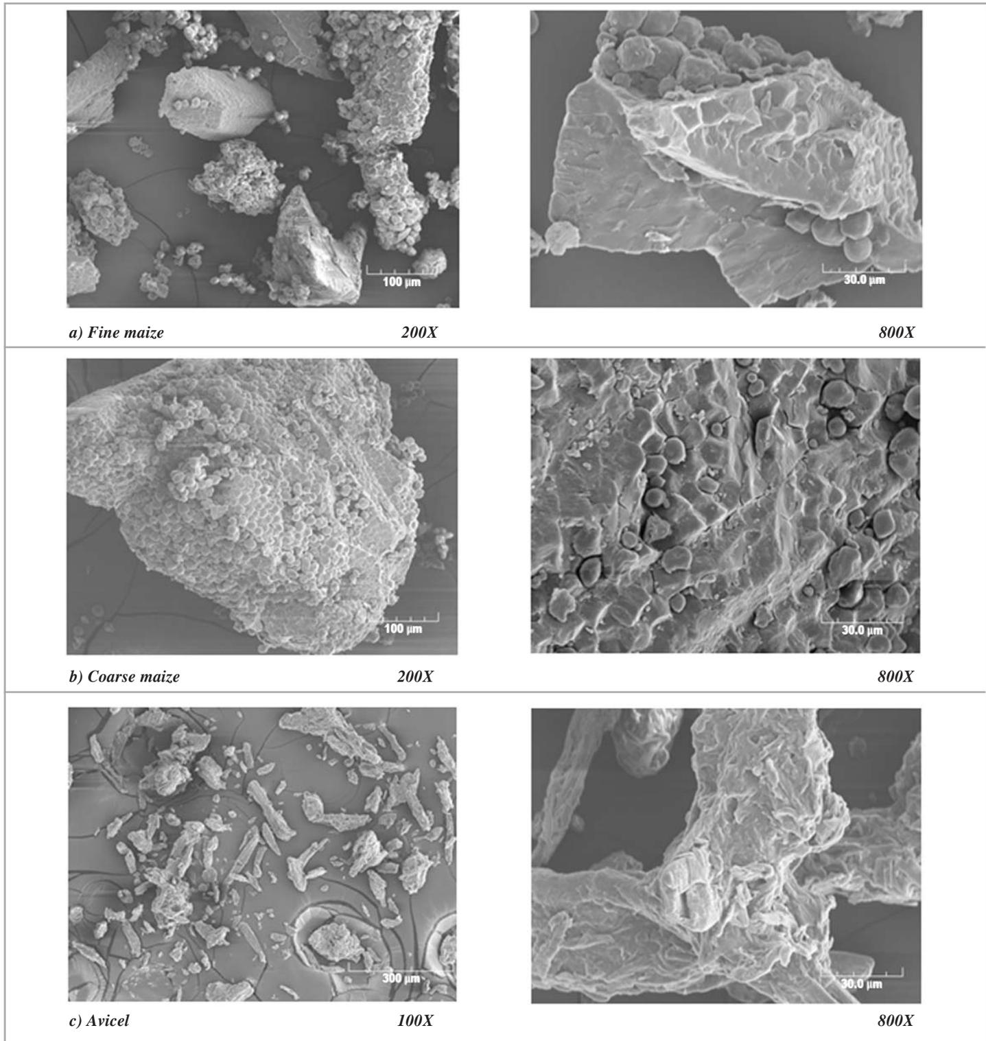
Figure 2: SEM images of (a) fine maize, (b) coarse maize, and (c) Avicel
