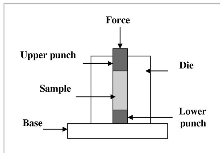
Figure 1: A schematic diagram of uniaxial die compaction
