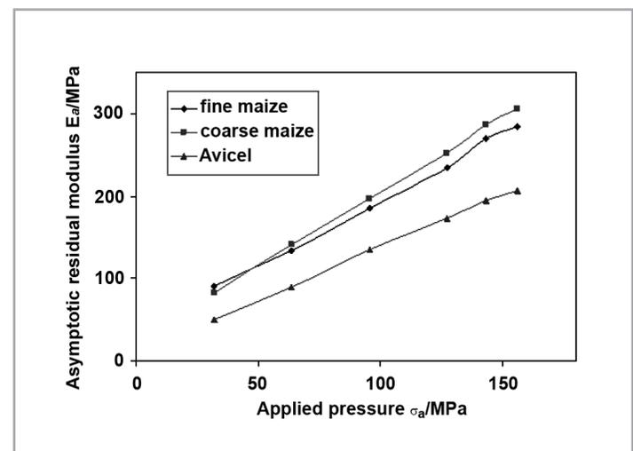
**Figure 7: The asymptotic residual modulus as a function of applied pressure. The lines are the trend lines**
