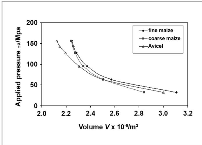
Figure 4: Applied pressure-volume relationship of powders at ambient conditions. The lines are the trend lines
