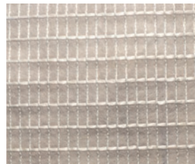
Non-woven geotextiles reinforced with high tenacity polyester yarns are used to strengthen and drain fine-grained clay soils
