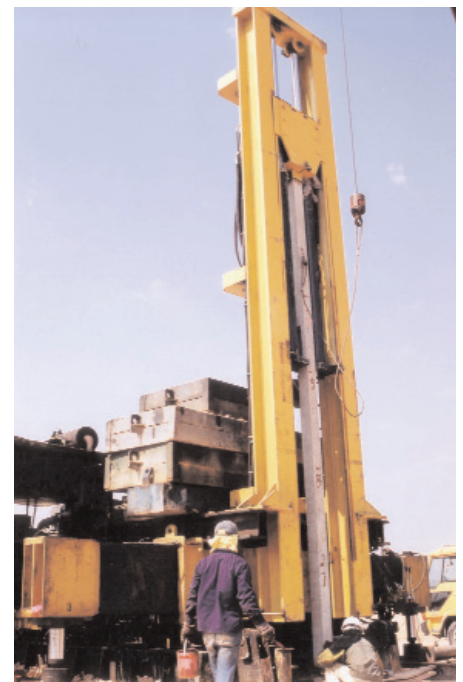
Figure 2 : Injection machine, environmental friendly with less vibration and low noise (courtesy of Soilmech Engineering)
